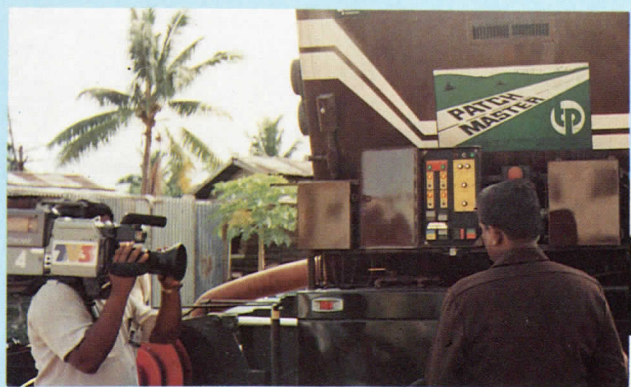
→ Patch Master is an advanced all-in-one road maintenance machine with remote control. It is excellent for pothole, truck, depression and surface crack repair. It was featured in TV3 recently.
