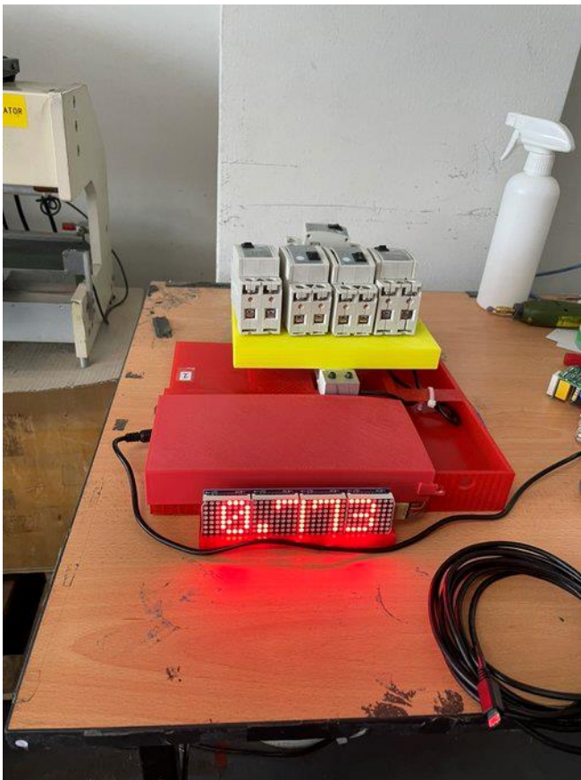
Prototype of IoT applications for monitoring production output in real time: IoT Weighing Scale System
